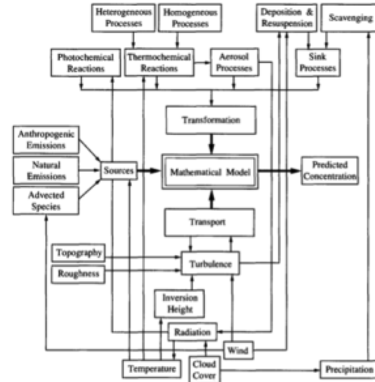
FIGURE 25.1 Elements of a mathematical atmospheric chemical transport model.
